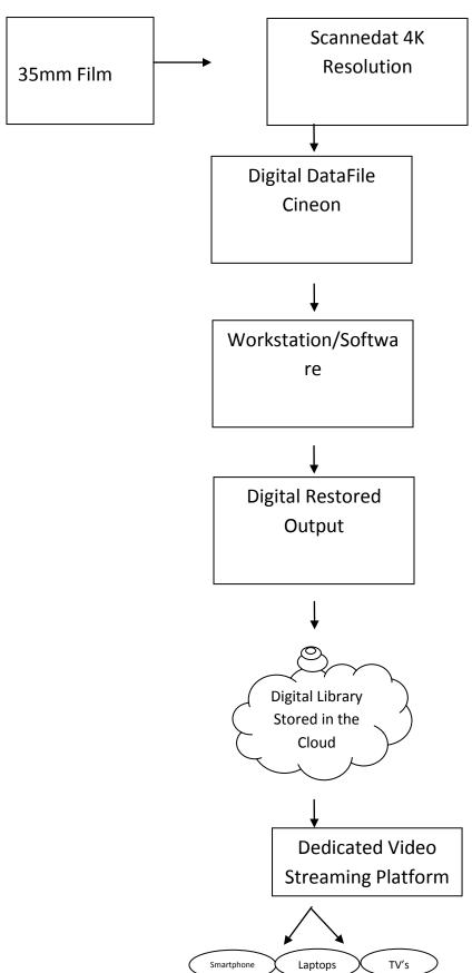
Note: In Workstation/software color grading is done at this stage in order to suit the mood of the movie and also removal of dust, dirt, scratches, stains and flickers. In addition to this Image stabilization is done. Sound quality is improved by our sound department separately.
